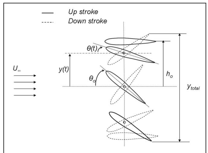
Figure 2: Airfoil undergoing combined plunging and pitching motions
