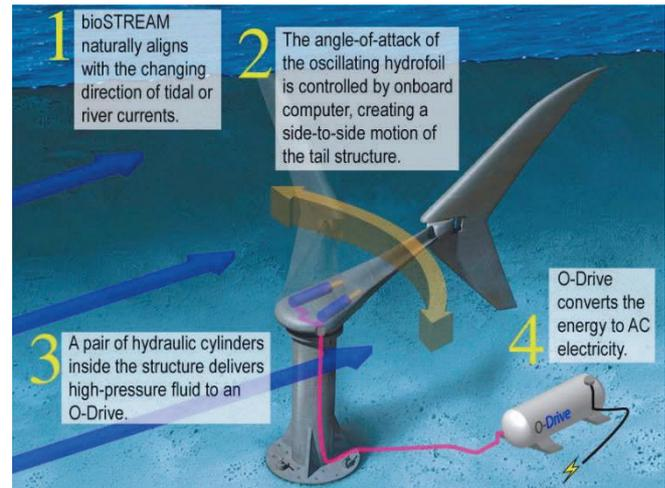
Figure 6: Fully flow driven flapping wing power generator (BioPower Systems 2019).
