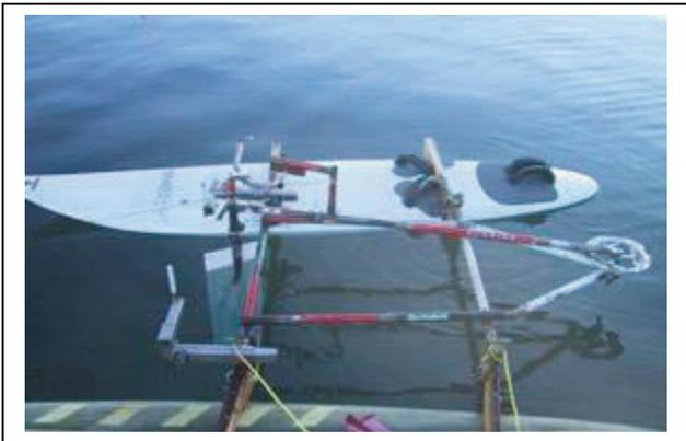
Figure 5: Fully flow driven flapping wing power generator (Platzer et al. 2009)
