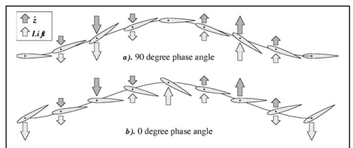
Figure 1: Bending-torsion airfoil flutter
