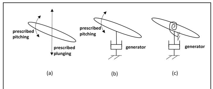
Figure 3: Schematics of flapping wing power generation systems (a) prescribed pitching and plunging motion (b) semi-flow driven motion and (c) fully flow driven motion
