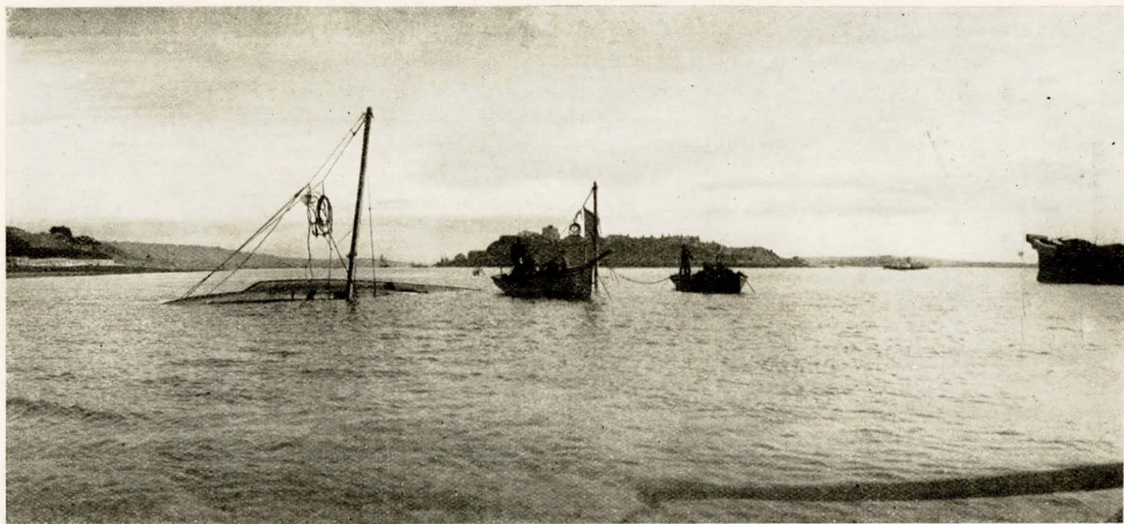
Fig. 1. Salvage of the Steamer Fleswick by Compressed Air. Before lifting.
