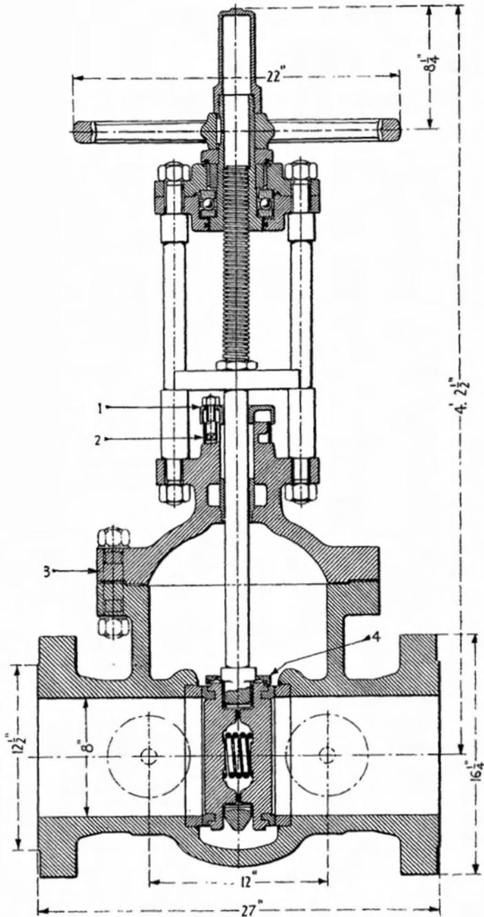
FIG. 1.—PARALLEL SLIDE VALVE
