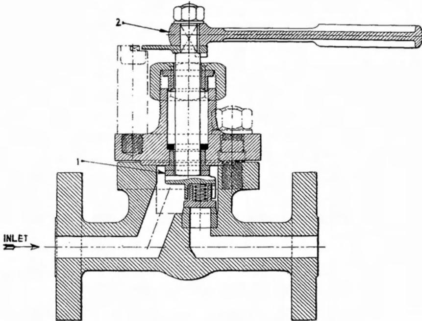
FIG. 2.—SMALL HIGH PRESSURE VALVE
