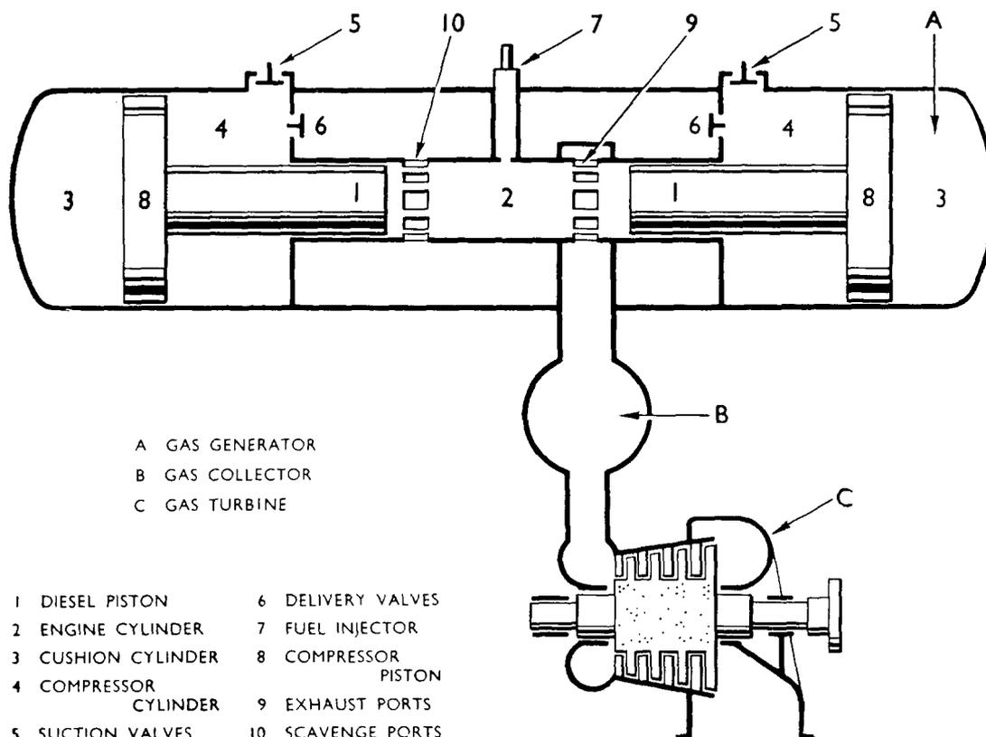
FIG. 1—DIAGRAM OF A FREE-PISTON ENGINE
