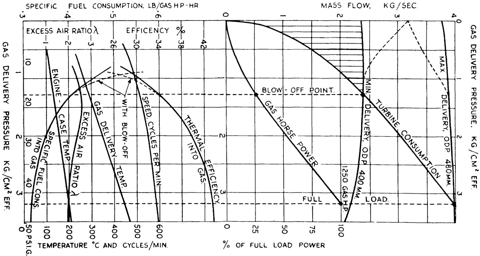
FIG. 3—CHARACTERISTICS OF A G.S.-34 GAS GENERATOR
