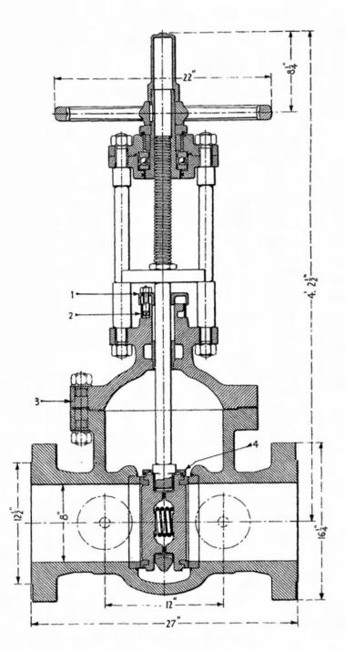
FIG. 1.—PARALLEL SLIDE VALVE
