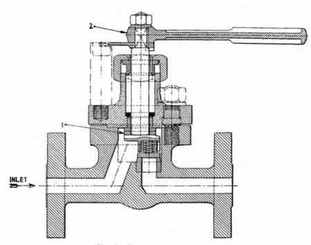
FIG. 2.—SMALL HIGH PRESSURE VALVE
